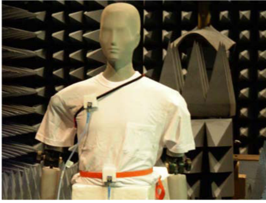
Fig. 1. Position b with the transmitting antenna in the belly and receiving antenna in the shoulder.
