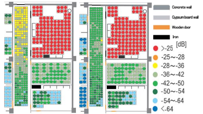
Fig. 3 Measured electric-field intensity Left: 2.45 GHz, Right: 5.2 GHz
